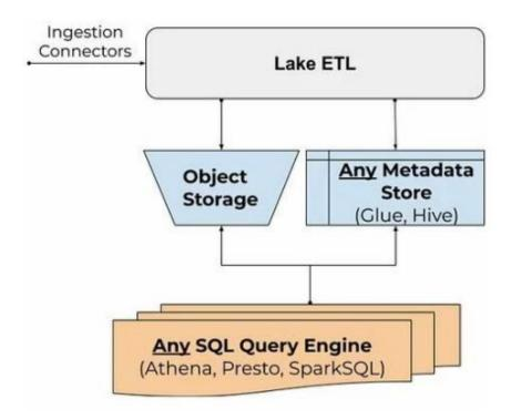
The challenge for data lake ETLs is how to keep the table-data consistent in real-time for queries while maintaining good performance. This is how Upsolver does it (using Athena as an example of a query engine):
